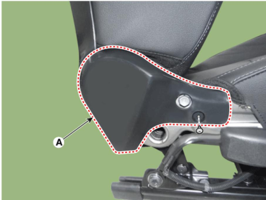
6. Remove the front seat back board lower protector (A).
