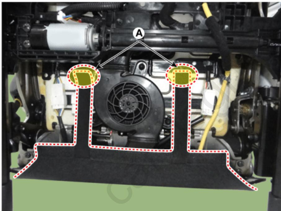
7. Disconnect the front seat cushion connectors & wiring mounting clip (A).
