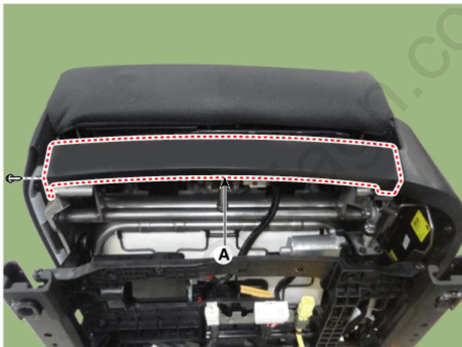
3. Remove the front seat outer shield cover (A) by using a remover.
