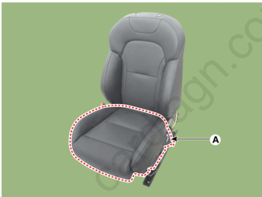
11. Remove the front seat cushion cover (C) from the front the seat cushion frame after removing the velcro tape (A) and hog-ring clips (B).
